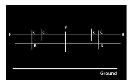
NOTE The visual aim procedure for lamps listed above as "N/A, do not measure downward" does not require the lower B-B horizontal line. Simply connect your +C marks with a horizontal line.
