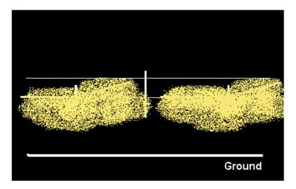
After adjusting a high/low beam headlamp in the low beam mode, do not attempt to readjust it in high beam mode. All high/low beam headlamps are meant to be adjusted on the low beam setting only-the high beam adjustment is correct when the low beam adjustment is correct. If you are experiencing a problem where setting the low beams correctly places the high beams too high, but setting the high beams correctly places the low beams too low, you are dealing with a poorly-designed headlamp.
